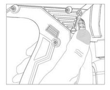
The volume of the material will be adjusted by turning the flow regulator screw.
