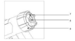
The airflow generated by the motor fan flows into the paint gun. The air flow serves to atomize the coating material at the nozzle and to pressurize the container.
